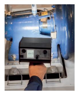
The SKF TKRS 41 is designed for general maintenance tasks and with its standard operating mode is streamlined for fast and straightforward usage. The professional mode can be activated for more demanding applications, for example when enhanced input signal modification is needed to trigger the stroboscope with machine signals. For convenience, the "SLOW" function can be used to examine all parts of the rotating machine in slow-motion.
